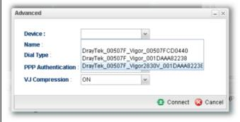
Specify the CPE from the Device drop down list; choose the name of the CPE; select PPTP or IPsec as the Dial Type; choose PAP\_only or PAP\_or\_CHAP as PPP authentication; enable or disable VJ Compression; then click **Connect** to build the VPN connection.
