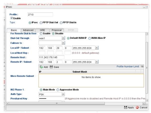
Type the Pre-shared key and choose a WAN Profile. Specify Local IP/Subnet Mask with 192.168.29.0/24. The Remote Host should be Vigor 2710's WAN IP address; And the Remote IP/Subnet Mask should be 192.168.2.0/24.
