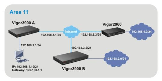
OSPF can place each router (e.g., Vigor3900A, Vigor3900B and Vigor2960 shown above) at the root of a tree and calculate the shortest path to each destination according to the cumulative cost to reach the destination.
