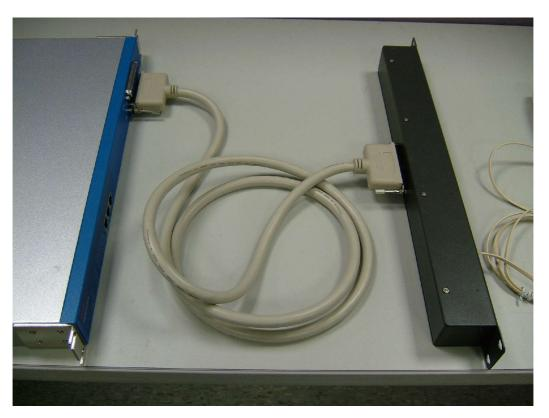
(1U Front Patch Panel to ADSL Modem)
