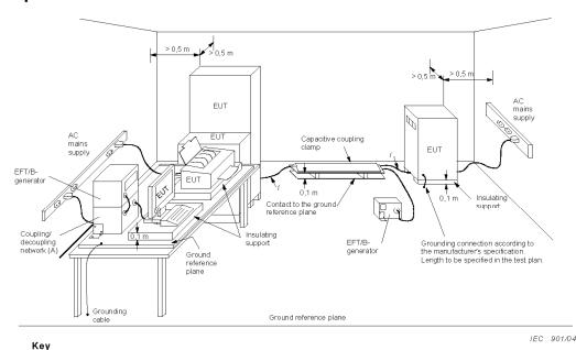
I length between clamp and the EUT to be tested (should be  $0.5 \text{ m} \pm 0.05 \text{ m}$ )
