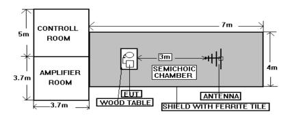
NOTE: The SPORTON 7m x 4m x 4m semi-anechoic chamber is compliance with the sixteen point's uniform field requirement as stated in IEC 1000-4-3 Section 6.2.
