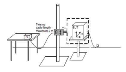
EUT: Equipment under test G: Test Generator
