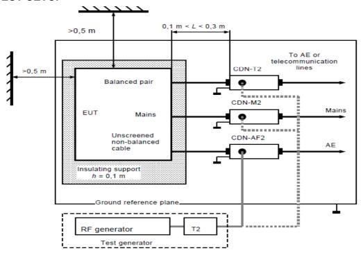
Note: 1. The EUT is setup 0.1m above Ground Reference Plane
