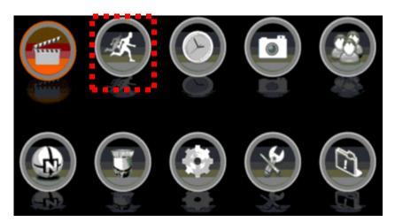
There are two types of events. First is the motion event which detects the movement in each camera. Second is the alarm event which detects the alarm input from alarm sensors. Users can adjust the alarm duration (in other word the record time) for the detected event.
