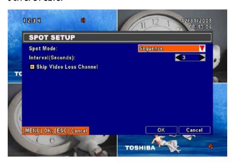
The DVR has two modes of video output; one is main video output, the other is spot video output. SPOT setup is for controlling the order of channels the system cycles through in SPOT mode. User can monitor every channel in the SPOT mode.
