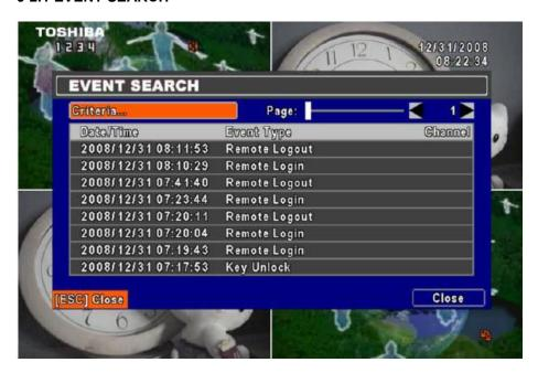
The DVR automatically records events with type, time and channel information included. If there is recording data for an event, the recording signal will be shown on the left side of time information. Rest your cursor under the line and press "ENTER", or left click your mouse to playback the recording data.
