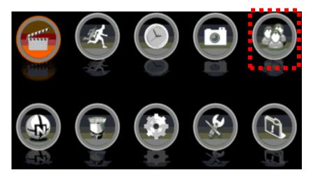
The Account Setup menu is used to provide role-based permission independently setting for each user (maximum of 4 users) to access DVR over network. The default admin account is  $\lceil \text{admin} \rfloor$  and password is "123456". You can register new accounts for users by setup user name, password, permission list, and **remember to click on the No.** to activate the account,
