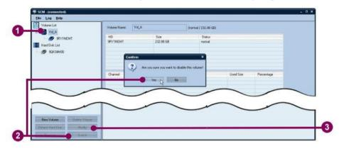
Figure 3-6 Add a hard disk to an existing volume
