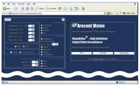
Figure 6-6 The camera setting provided by the manufacturer Some tabs will show the live image of the channel. An IP address is above the live image. Click the IP address, and a browser will be opened to shows complete camera settings.
