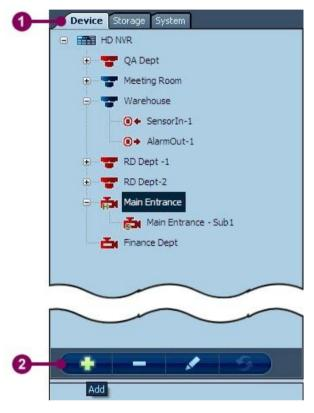
Figure 6-7 Add a channel manually
