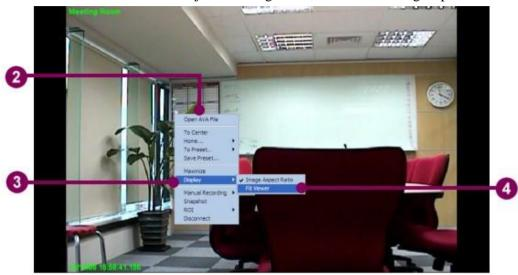
Figure 4-22 Adjust the image ratio
