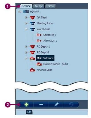
Figure 6-8 Add a channel automatically
