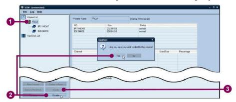
Figure 3-7 Remove a hard disk from an existing volume
