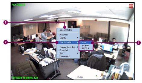
Figure 4-41 Switch the codec on playing
