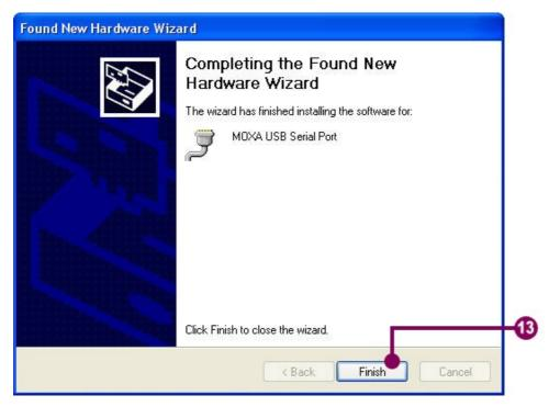
**13.** When the MOXA USB Serial Port driver is installed, click 'Finish' to continue. When the wizard is done, DO NOT restart the system.
