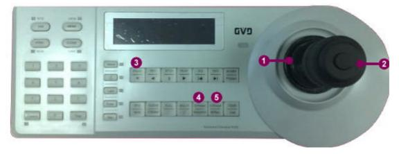
Figure 5-3 Function keys of PTZ mode
