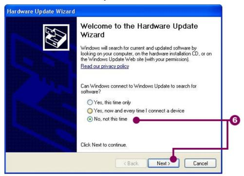
**6.** As soon as the RS-485 converter is plugged, the system will detect automatically the device driver. If no available driver is found, the system activates the Found New Hardware wizard. Click 'No, not this time' item in the hardware update wizard and click 'Next'.
