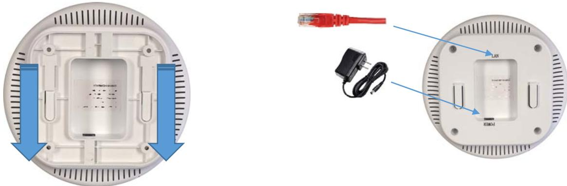
Connect an Ethernet cable to the RJ45 LAN port on the access point. Connect the other end of the cable to either a PoE injector (which connects to your network), a regular LAN switch.
