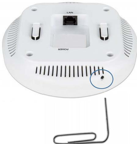
Use a sharp object like a paper clip to push in the reset button. Do that for about 6 seconds while the device is powered on and the access point will automatically restore the factory settings and restart.
