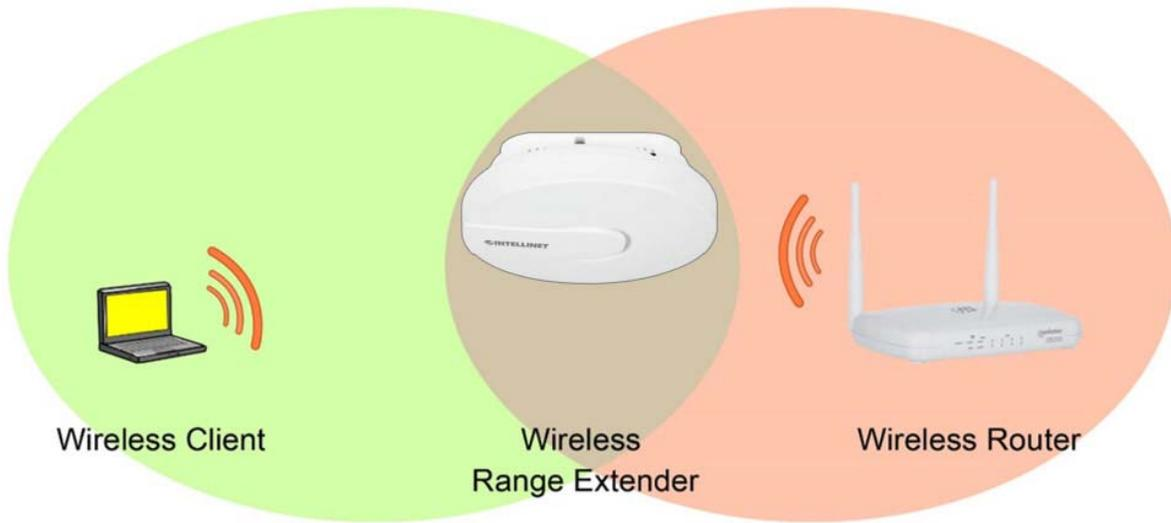
A wireless repeater (also called wireless range extender) takes an existing signal from a **wireless router** or wireless access point and rebroadcasts it to create a **second network**. The effect is that the range of the wireless network is increased. The other function of the wireless repeater is that it creates a bridge to another wireless network for all clients that are connected to the LAN port on the access point. In summary, there are two functions that the access point needs to do:
