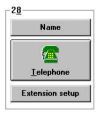
Below the button bar, you will see the display fields for the individual extensions (21..28). Via the buttons "Name", "Telephone" (this will show the current service identifier for the extension) and "Extension Setup" you can access the dialogue windows to alter these settings for the extension.
