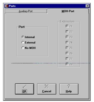
select in the field "Port" the point "External" and then select the extension to be used for the connection of the audio source. Afterwards connect an appropriate audio source (e.g., an Emmerich MOH-Module and an audio source) to the extension instead of the usual analogue terminal.
