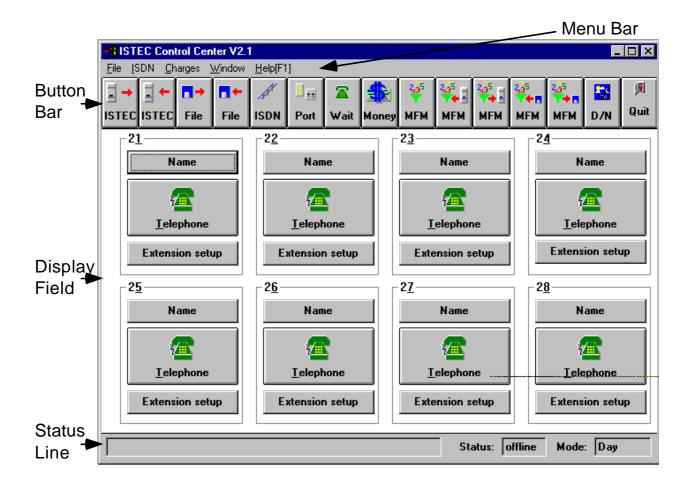
Figure 2-1: The ISTEC Control Center's Main Window
