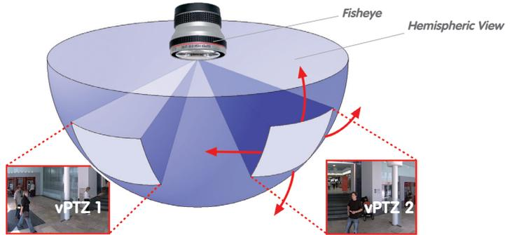
When ceiling mounted, the image area of the hemispheric camera covers the entire room. The image in the hemisphere is convex, particularly near the image borders. These image sections are corrected for the viewer by the integrated distortion correction software, allowing a view of the scene from the usual perspective. The **virtual PTZ feature** allows you to enlarge or move image sections within the hemisphere, just like a PTZ camera yet, with MOBOTIX, this is achieved with no moving parts.
