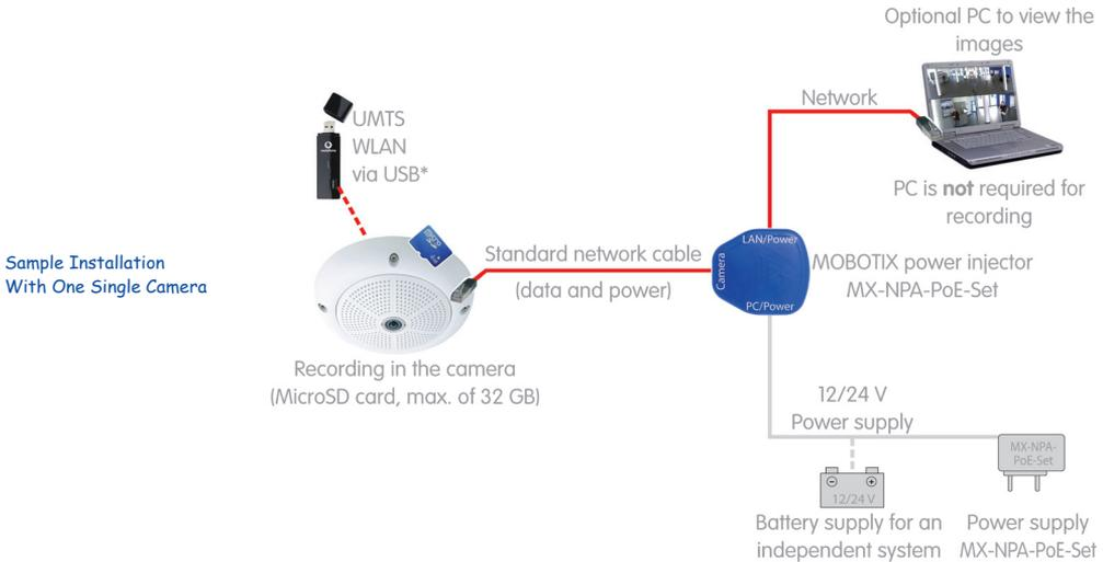
**Sample Installation with One Camera:** Power is supplied via a standard Ethernet cable using the MX-NPA-PoE set or using a battery (mobile surveillance solution).
