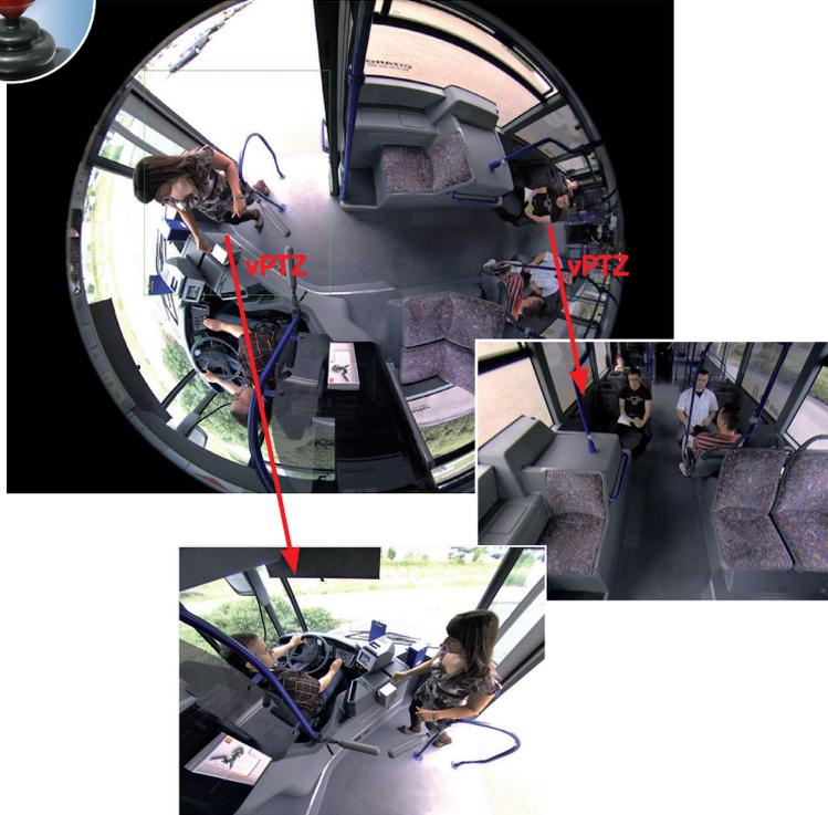
The vPTZ functionality works differently depending on the camera operation platform (**web browser, MxEasy, MxControlCenter**). Virtual zoom, pan and tilt using MxEasy and MxControlCenter is very simple thanks to special software tools and the use of an optional joystick. However, a joystick may also be used even with pure browser-based operation from Internet Explorer (together with an ActiveX plug-in).
