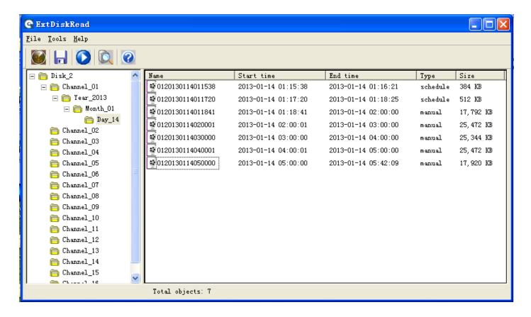
After connecting hard drive disk to PC. As we can see, tool can read the contents of the hard drive disk.
