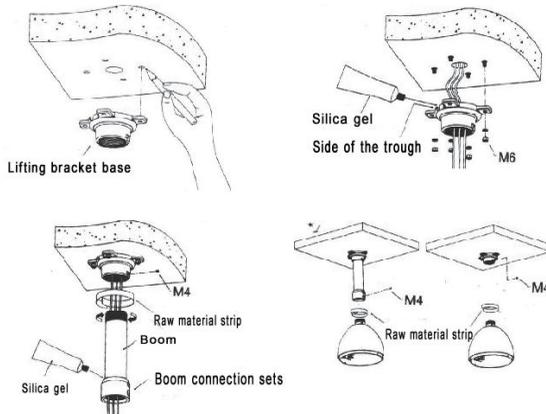
**Note: If the camera used in outdoor, Waterproof seal should be in the camera and bracket connecting part.**
