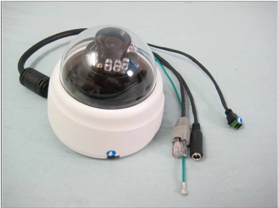
Discharge Point-1 (blue arrow shows air discharge)
