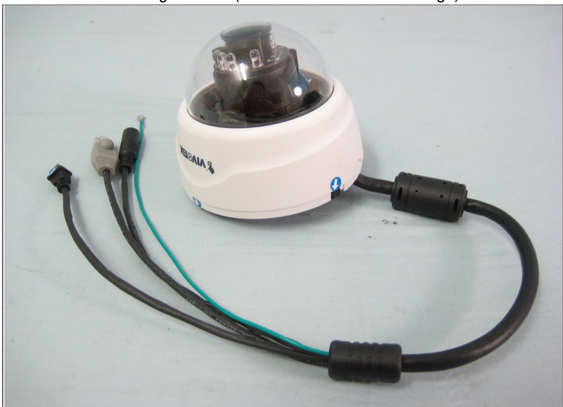
Discharge Point-2 (blue arrow shows air discharge)
