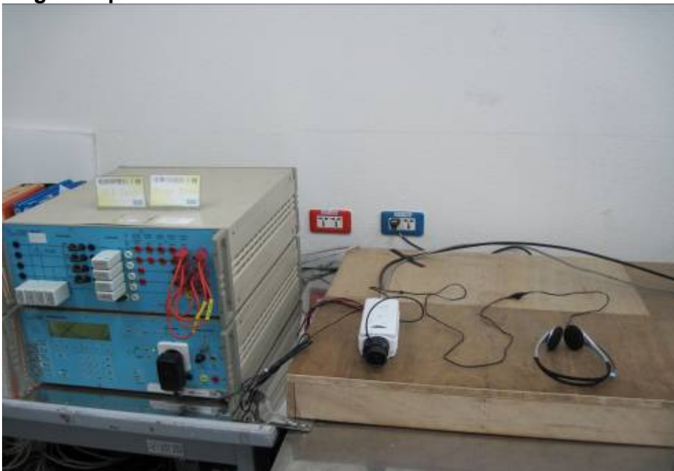
EFT Testing Set-up
