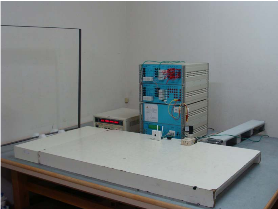
Voltage Dips Test Setup
