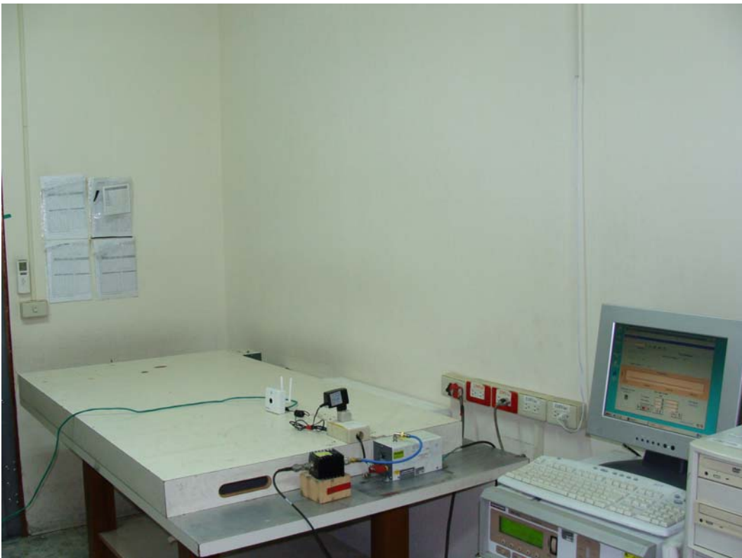
Conducted Susceptibility Test Setup
