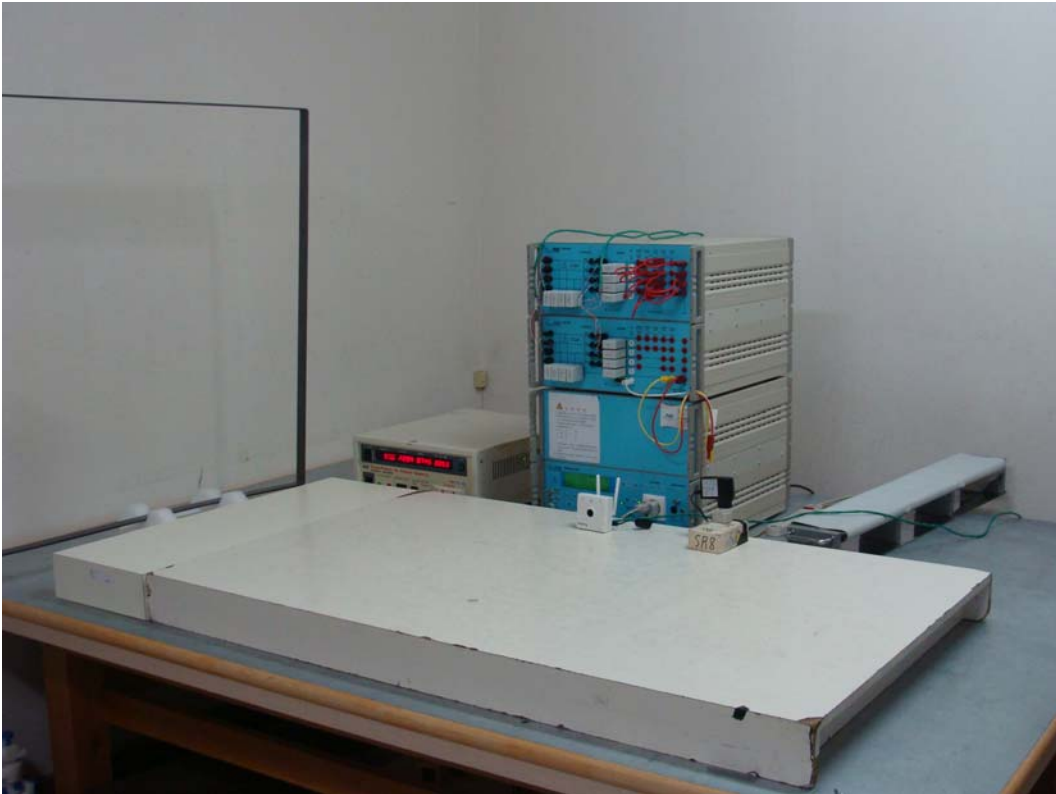
Conducted Susceptibility Test Setup
