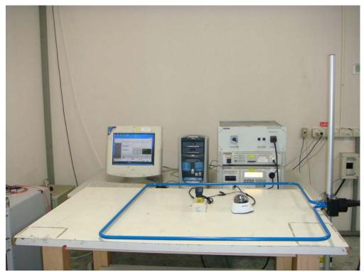
Test Mode : Mode 2: PoE Mode Description : Power Frequency Magnetic Field Test Setup
