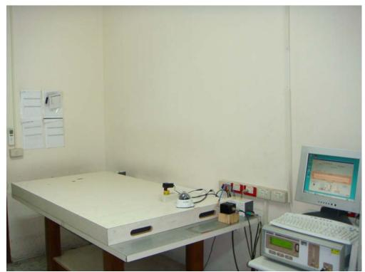
Test Mode : Mode 1: Adapter Mode Description : Conducted Susceptibility Test Setup - CDN
