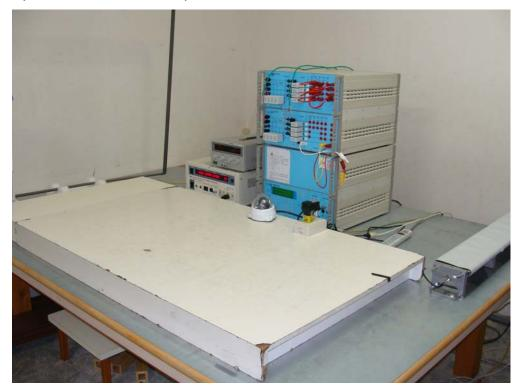
Test Mode : Mode 1: Adapter Mode Description : EFT/B Test Setup - Clamp
