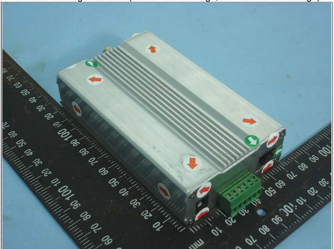
View of Discharge Point-2 (Green: Air discharge, Red: Contact discharge)
