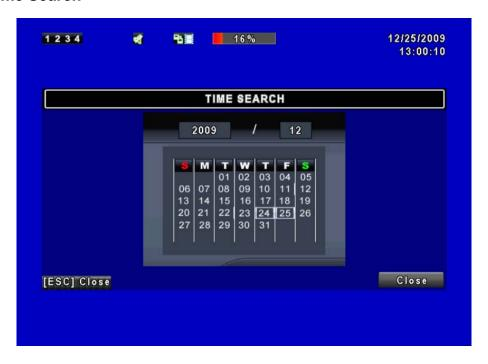
TIME SEARCH, you can search for a specific time of the recording data to playback. Dates with recording are shown by data marked with a red square [ ]. System will start playing back according to the date that you've selected. Calendar will be shown by using mouse to click on "year" and "month".
