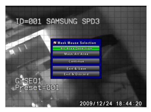
There are partitions in motion detection area. Under initializing status, motion detection area is in the entire screen. Red colored area is undetected; yet the detected area is transparent.
