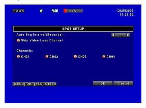
The DVR has two modes of video output; one is the main video output, the other is spot video output. SPOT setup is for controlling orders of channels that the system cycles through in SPOT mode. User can monitor every channel in the SPOT mode.
