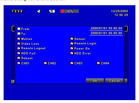
The amount of events can be numerous. Therefore, you can facilitate event sorting by setting up "criteria". Setup "start time" and "end time" for each event search, then the search result will be limited to this specific period of time. Only events and channels that are ☑ checked will be sorted in event search as well.
