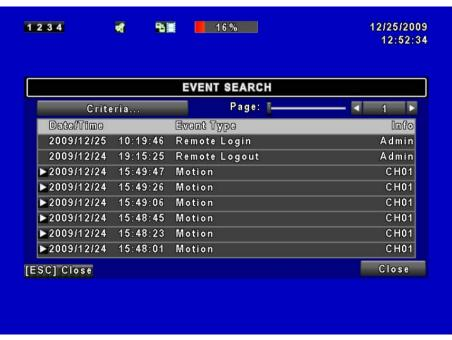
The DVR automatically records events with type, time and channel information included. If there is recording data for an event, a yellow signal icon will be shown on the left side of time information. Rest your cursor under the line and press "enter", or left click your mouse to playback the recording data.
