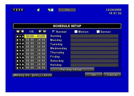
Apart from manual recording, you can also setup the recording time by weeks and schedule recordings include: normal, motion detection, and sensor detection.
