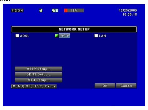
If the DHCP option is used for DVR network connection, an IP address is assigned by the DHCP server automatically.
