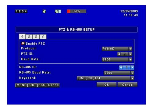
The DVR allows users to control PTZ functions of your camera. To enable PTZ function, the 485 cable should be connected to the RS-485 port of DVR.
