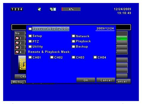
The Account Setup is set to provide individual user (maximum of 4 users) role-based permissions, including access to Setup menu, Network operation, PTZ function, Playback, Utility, Backup and Mask on specific channels while playing back.
