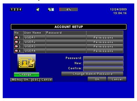
The Account Setup menu is used to provide role-based permission independently for each user (maximum of 4 users) to access the DVR over network. The default admin account is [admin] and password is "123456".
