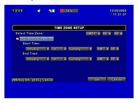
In time zone setup, users can change the time zone and activate Daylight Saving Time function according to your DVR location.
