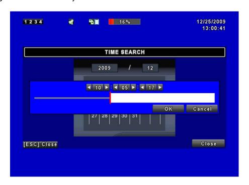
Click "date" to display recording time of that specific date with time bar. You can change time (hour/ minute/ second) or click on a specific time of time bar by mouse then press "YES". DVR will playback the selected recording data.
