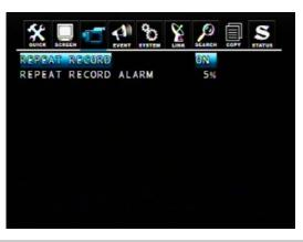
ON: When repeat recording, if the HDD is full, DVR will overwrite the recorded data automatically. OFF: Stop to record when the HDD is full.
