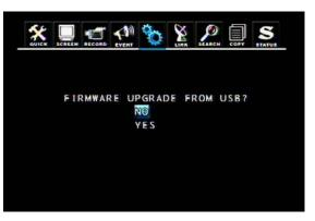
You can update the DVR firmware through the USB interface. Insert the USB device with the all.dvi file into DVR and press YES to update the firmware.
