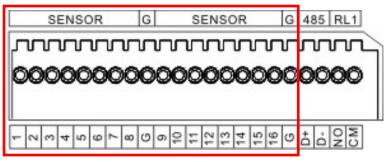
16CH: SENSOR 1~SENSOR 16 8CH: SENSOR 1~SENSOR 8 4CH: SENSOR 1~SENSOR 4
