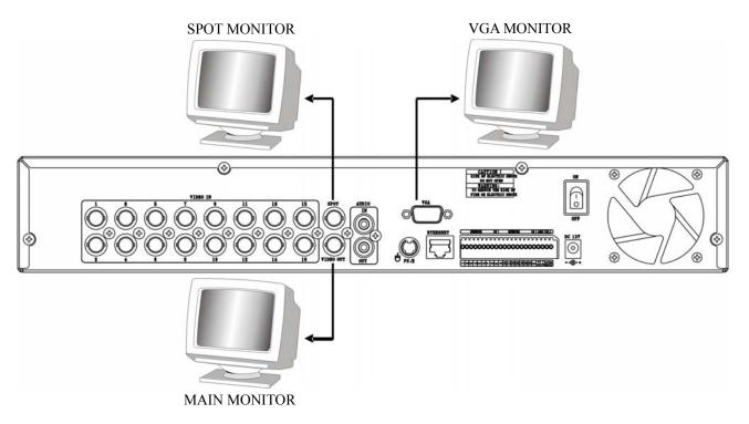
DVR supports two types of monitor output, one is Composite output (BNC connector); the other one is VGA output (DSUB-15). But you can just select one monitor output type at a time.
