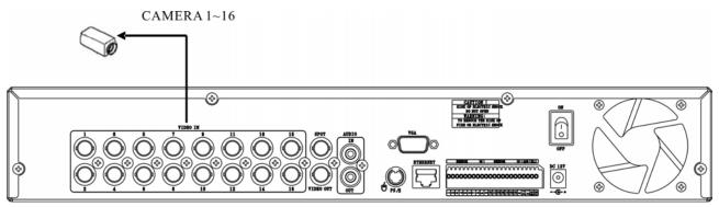
\* Connect a female BNC connector of each camera to a male BNC connector, "CAMERA IN" port.
