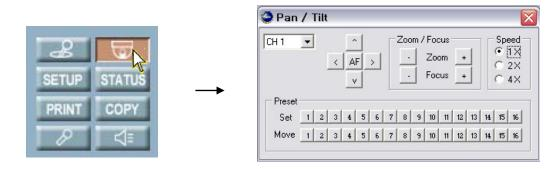
AF: AutoFocus Adjustment Zoom: PTZ camera Zoom in/Zoom out control Focus: PTZ camera Focus adjustment
