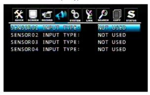
Select the right sensor type according to the type of installed sensor with the unit.
