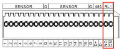
The relay device should be set to NO (Normal Open) and it will change to NC (Normal Close) when an event has been triggered.
