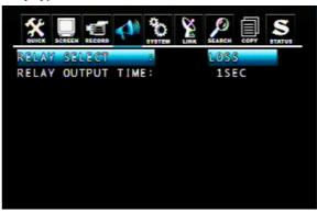
DVR provides a relay output interface; the following events will trigger off the relay signal:
