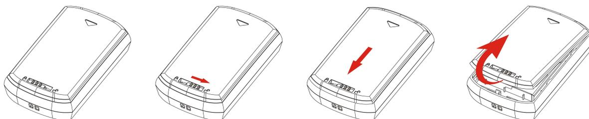
1.2 Insert the SIM card as the label indicated (metal contact face down).
