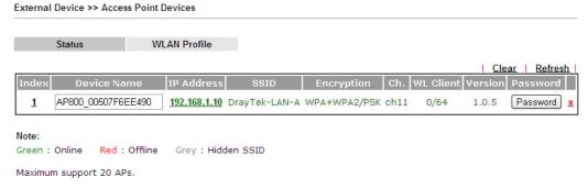
In this case, a device named with AP800\_00507F6EE4980 has been detected by Vigor router.
