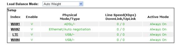
Note: The line speed setting of WAN interface is available only when According to Line Speed is selected as the Load Balance Mode.
