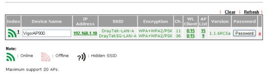
When AP Devices connect via an intermediary switch, please ensure that UDP:4944 port and the HTTP port of AP Devices are not blocked so that the AP status can be retrieved.
