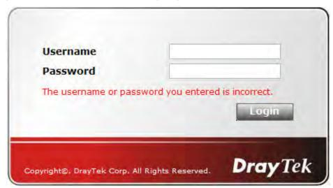
■ In above description, you access an external web site to trigger the authentication. You may also directly access the router's Web UI for authentication. Both HTTP and HTTPS are supported, for example http://192.168.1.1 or https://192.168.1.1 . Replace 192.168.1.1 with your router's real IP address, and add the port number if the default management port has been modified.
