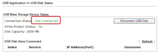
Note: If the write protect switch of USB disk is turned on, the USB disk is in READ-ONLY mode. No data can be written to it.
