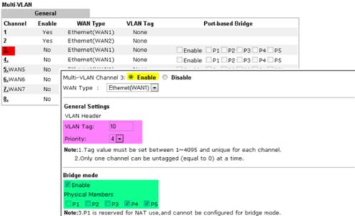
Set-top box (STB) or the other kinds of media devices are able to attach with Port4 or Port5 of LAN. Those devices that attached with Port4 or Port5 are able to access the services network directly which your ISP provided.
