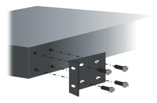
After the bracket installation, the Vigor3910 Series chassis can be installed in a rack by using four screws for each side of the rack.
