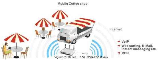
After connecting into the router, 3G USB Modem will be regarded as the second WAN port. However, the original Ethernet WAN1 still can be used and Load-Balance can be done in the router. Besides, 3G USB Modem in WAN2 also can be used as backup device. Therefore, when WAN1 is not available, the router will use 3.5G for supporting automatically. The supported 3G USB Modem will be listed on Draytek web site. Please visit www.draytek.com for more detailed information.
