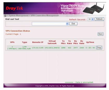
The remote IP and virtual network IP addresses (assigned by local router) will be displayed on the **VPN Connection Status** page.
