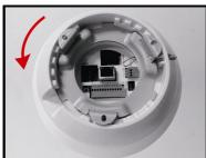
Tighten the screw at the side of the Fixing Plate. Finishes install Camera on T-Bar Bottom Mount.
