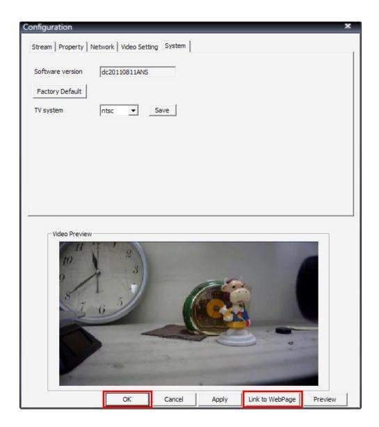
If users wish to connect to the IP camera's webpage via a browser, click <Link to WebPage> at the bottom. When the setting is completed, click <OK> at the bottom to exit the Configuration Menu.
