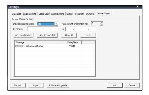
Next to <DeviceWizard Status>, select <ON>/<OFF> to enable/disable the Device Wizard function. If the Device Wizard function is enabled, setup white and black lists via specifying IP range. <Max count of connect fail> allows users to choose how many times VSS will try to connect an IP camera. After the specified number of tries and VSS is still unable to connect an IP camera, IP address of the IP camera will be automatically added to the black list.
