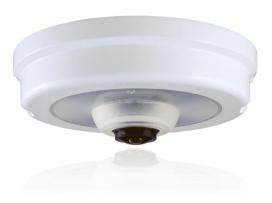
The Full HD Multiple Streams Fisheye IP Camera is a high resolution surveillance solution featuring 360 Degree Panorama View that allows users to monitor a wide angle surveillance environment without blind spot with just one camera. The camera not only delivers clear images through multi-streaming video, its lens with up to 5 Mega-pixel high resolution image also provides panorama function with quad view that enables four different assigned angles images to display simultaneously for monitoring.
