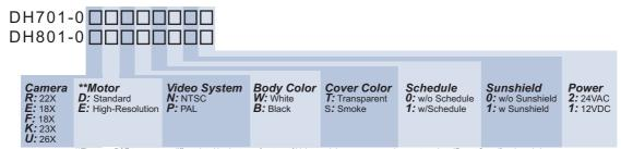
\*\*There are D&E type motors, differentiated by the type of motors of high speed dome cameras and presents various "Preset Speed" and resolutions Standard Resolution: 768 steps/circle. High Resolution: 1600 steps/circle
