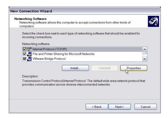
In TCP/IP address assignment, if the PC has DHCP server, then choose <Assign TCP/IP addresses automatically using DHCP>, else choose <Specify TCP/IP addresses> and enter the range of IP addresses that users wish to use. Once done, click <OK> to confirm and back to Networking Software menu. Click on <Next> to continue.
