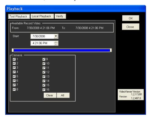
In the <Tool Playback> tab, users can set starting time and displaying cameras of the selected video. Then click <OK> on the upper right-hand corner of the window to start playback the video with selected starting time and displaying camera on the main window.
