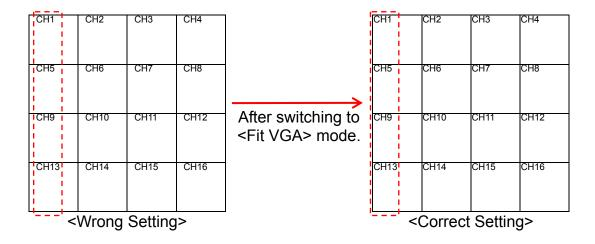
PC Monitor is used in the example above. In the <Wrong Setting>, the Title Position is set to <Fit BNC> instead of <Fit VGA>. Since it is not the right setting, the titles of CH1, CH5, CH9, and CH13 are slightly shifted toward the center screen of each channel. After switching to <Fit VGA>, the titles have been shifted back to the proper position as shown in the <Correct Setting>.
