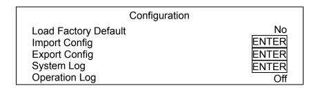
Also under the Configuration setup menu, set <Operation Log> to <On> and operation logs will start to be recorded in the system log. Alternatively, set to <Off> and operation logs will not be part of the system log.
