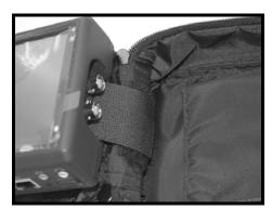
Pull the strap through and stick it tightly across the case joint to the Velcro on the opposite side.
