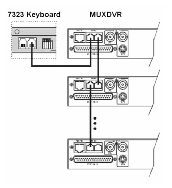
If you turn on power (with adapter) or connect 7323 with RS485 cable, the keyboard (7323) will automatically search MUXDVR that connected with 7323 by RS485 cable. The channel LED will be lighted one by one during search period. The action will be continued until 7323 has received any response from anyone MUXDVR. The channel LED corresponds to the responsive MUXDVR will be flashed.
