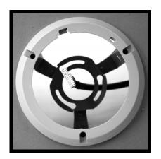
Mount the Dome Camera onto the In-Ceiling Mount with the exact orientation as indicated. Firstly, align the fixing screw hole on the Lock Bar with the mating slot on the ring of the In-Ceiling Mount. Then rotate the camera clockwise, and let the screw hole on the Lock Bar align with the fixing screw hole on the In-Ceiling Mount's ring.
