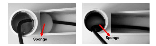
**5)** Thread the cable(s) through the Indoor Mount Kit and join the Indoor Mount Kit to the Compact Pendent Mount with the supplied screws and washers. Then adjust the Waterproof Rubber to the joint.
