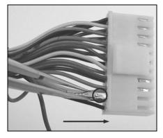
To unlock the terminal, press the hook, as indicated in the figure, with a proper tool and pull it out gently.
