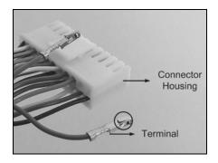
Insert the terminal into the pin holes on the connector housing, with the hook outward, as indicated in the figure.
