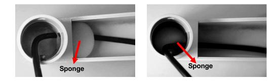
**5)** Thread the cable(s) through the Outdoor Mount Kit and join the Outdoor Mount Kit to the Compact Pendent Mount with the supplied screws and washers. Then adjust the Waterproof Rubber to the joint.
