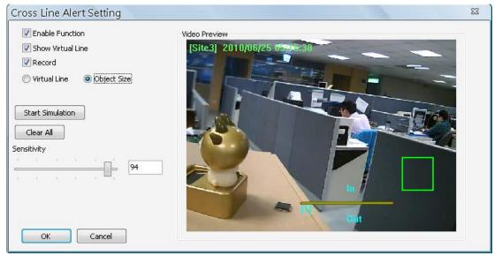
Enable Function: Check on it to enable cross line alert function.
