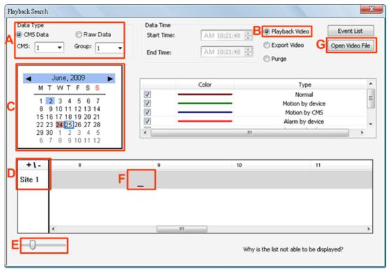
Step A. Select <CMS Data> and choose CMS server & group. Alternatively, select <Raw Data> and allocate a folder containing DVR/NVR HDD files. Step B. Select < Playback Video>.
