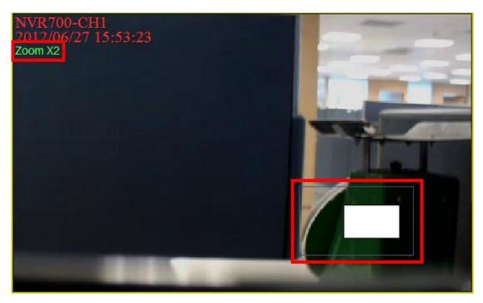
On the upper left-hand corner will show zoom-in multiple. The maximum multiple is X7. Also on the lower right-hand corner will show the position of current viewing area, shown as an inner white rectangle, compared with the original screen, shown as an outer rectangle frame.
