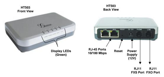
The HT503 has one FXS port and one FXO port. The PHONE port next to the power supply is an FXS port. The LINE port on the back right of the HT503 is an FXO port. Both the FXS port and the FXO port can have a separate SIP account. This is a key feature of HT503 as it supports simultaneous calls on both the FXS port and FXO port. Telephone calls can be originated from or terminated on the PSTN network remotely via the FXO port.
