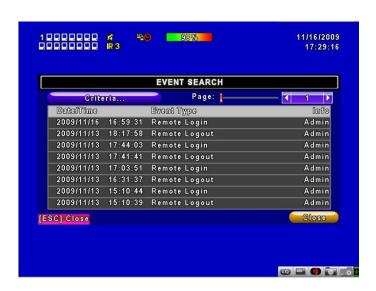
The DVR automatically records events with type, time and channel information included. If there is recording data for an event, a yellow signal will be shown on the left side of time information. Rest your cursor under the line and press "enter", or left click your mouse to playback the recording data.
