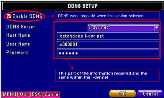
**Step 5.**Back to the i-dvr.net, on this page by pressing "F5: Refresh", IP will be automatically updated into the DVR of the real IP location.
