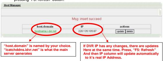
**Step 4.** Enter DVR  $\rightarrow$ Main Menu  $\rightarrow$  Network Setup  $\rightarrow$  DDNS. Activate DDNS functions and input related information.
