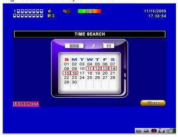
Click "date" to display recording time of that specific date with time bar. You can change time (hour/minute/second) or click on a specific time of time bar by mouse then press "**ok**". DVR will playback the selected recording data.
