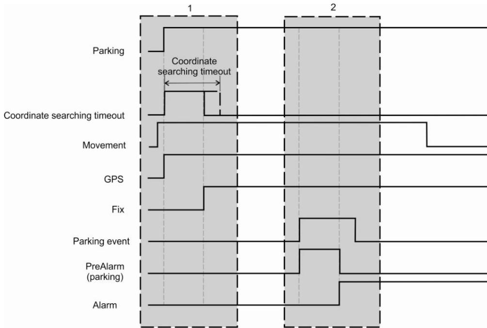
Operation of parking function, when new coordinates are found by the time device leaves parking zone and comes back after *PreAlarm* time. There was movement at first.
