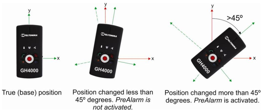
*Man – down* function is enabled and device position is changed more than 45 degrees *PreAlarm* is activated. If device goes back to its true (base) position until *PreAlarm* time runs out – alarm is not activated. Device continues monitoring its position.
