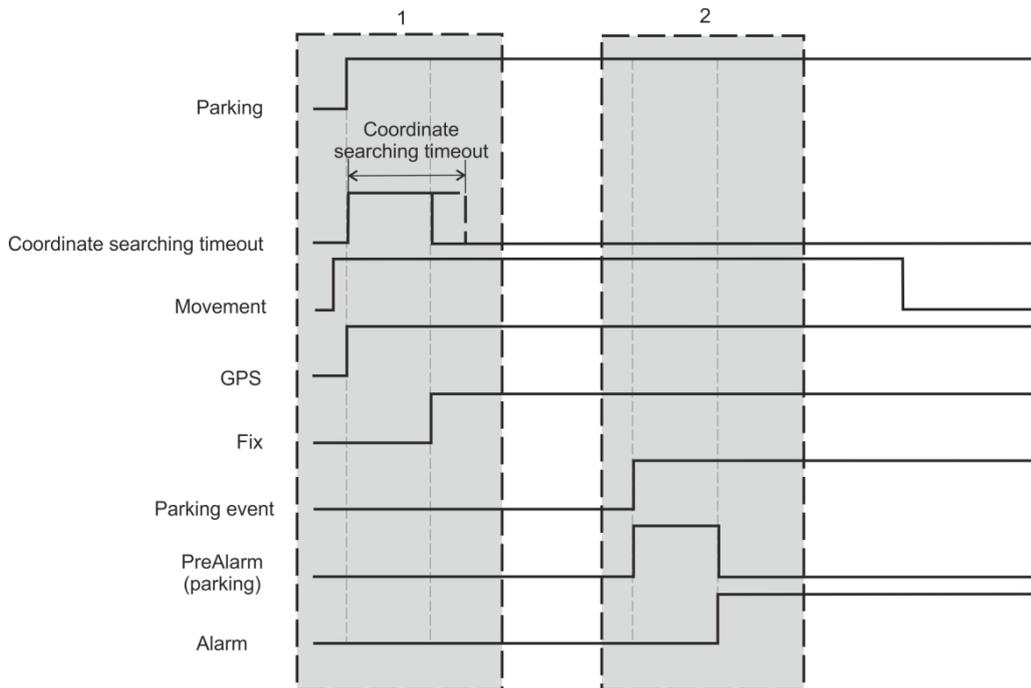
Operation of parking function, when new coordinates are found by the time device leaves parking zone and does not come back. There was movement at first.
