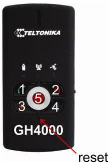
Configurable buttons are numbered in the picture. The reset button is shown with the arrow. It can be pressed only with something long and sharp like paper clip. Lock switch is located on the right side of device.
