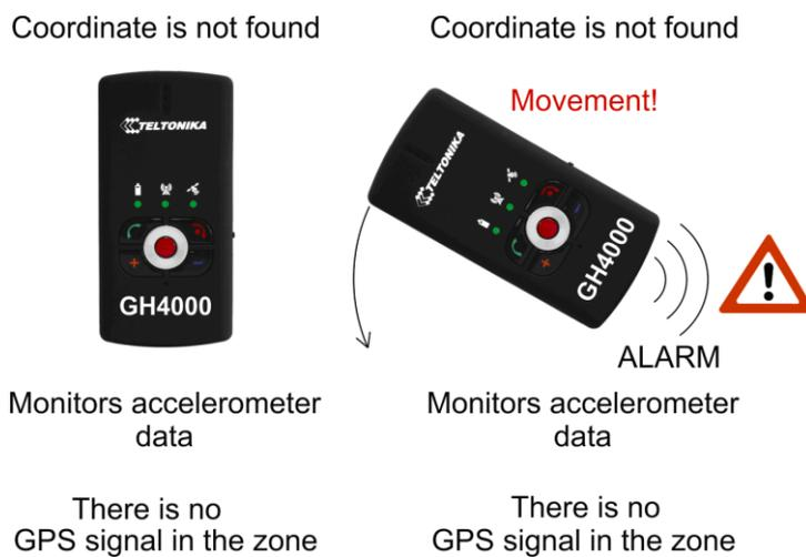
Parking function is activated. There is no movement. GH4000 does not find new coordinate. Device goes to movement (accelerometer) monitoring mode. PreAlarm is activated when movement is recorded. Alarm is activated after PreAlarm time runs out. Couple scenarios, when device is not able to get new coordinate, are displayed below.
