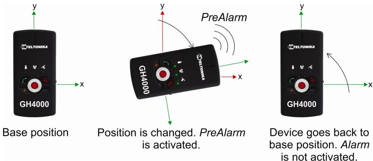
When *Man – down* function is enabled and device position is changed more than 45 degrees *PreAlarm* is activated. Device does not go back to its true (base) position until *PreAlarm* time runs out – alarm is activated.
