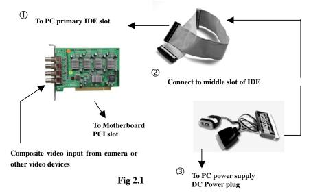
Connect video signals to the camera input ports of VP-40. These signals can be Camera, VCR, TV or VCD/DVD player as long as they are NTSC/PAL compatible composite videos.
