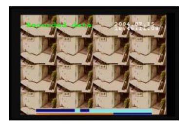
**GPI** - The screen shows where alarm triggers were generated. The red bar shows the triggers. To move to the next motion detection or alarm trigger event, press the Right/Left arrow buttons.
