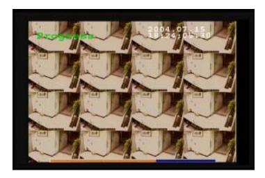
**Recorded Data -** The aqua colored line represents how much of the one hour time interval was recorded. A full blue line means that the whole hour interval was recorded.
