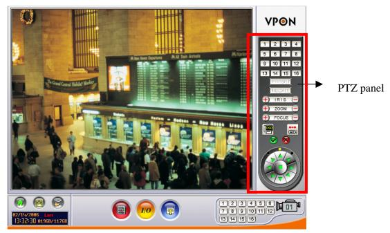
PTZ panel: You can do preset and recall, zoom in/out, focus, iris control to current camera.
