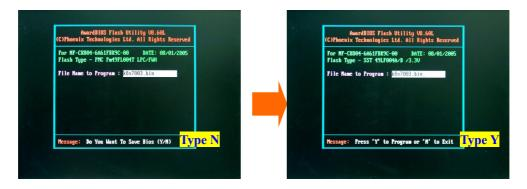
The next screen (shown above-right) will display a message "Press 'Y' to Program or 'N' to Exit". Then type 'Y' to begin the onboard BIOS flash procedure.
