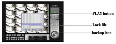
The alarm condition which caused the file to be recorded is indicated in the list. For instance, in the screen shot shown here, the letter **M** next to a file indicates that the file was recorded after motion was detected by the camera. Pick a recording from the displayed list and click **OK** to play. The recording will play on screen. Click the **LIVE** button to return to live images from the connected cameras.
