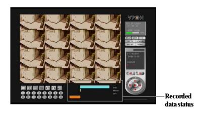
The moving orange line indicates the current playback status. Click anywhere on the **Data**, **Motion**, or **GPI** lines to start playback from the required point.
