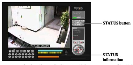
The status panel displays the playback status of the current recording. The aqua line (**Data**) indicates recorded data over a one hour time interval. The yellow bars (**Motion**) indicate the instances when motion was detected. The (**GPI**) indicate when a GPI event was detected. The moving orange line indicates the current playback status. Click anywhere on the **Data**, **Motion**, or **GPI** lines to start playback from the required point.
