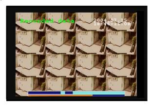
Recorded Data – The aqua colored line represents how much of the one hour time interval was recorded. A full blue line means that the whole hour interval was recorded.
