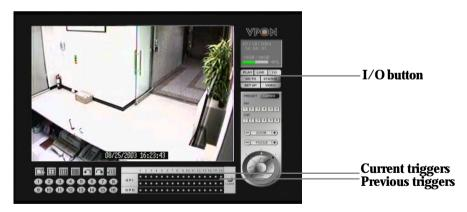
When an alarm has been triggered, the GPI and GPO that are connected will show the status of the input or output device. GPI devices will show **NC** (normally closed) or **NO** (normally open) as the status of the switch while GPO devices will show **On** or **Off** as their status.
